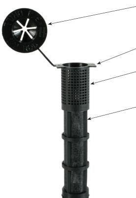
Integral Cap: Serves to center and secure the rod in the screen tube, while displaying important information such as rod diameter, drill bit diameter and the Simpson Strong-Tie® "≠" symbol for easy inspection after installation. The cap also prevents adhesive from running out the front of the screen tube.
