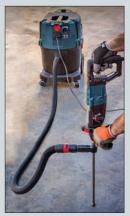
Bosch / Simpson Strong-Tie DXS drill bit used with the vacuum dust extraction system.
